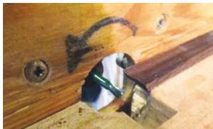
▲ Pic B. The same cutter, left at the same depth of plunge, is lowered to shape the sides of the spline – this time without the sled. Tony routs a long length at a time, then cuts it into slices and slides each slice with glue into a corner slot
